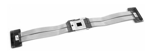
This guide shows you how to install the interposer between the microprocessor and the socket on the system board.
