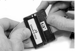
**18** Optional: install the supplied nylon screws to keep the paddles on the end of the analysis probe cables for additional retention.
