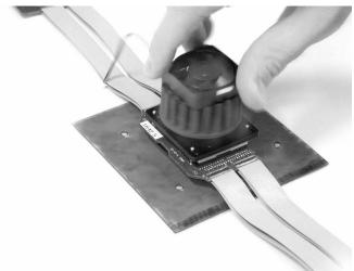
Tip: Rotate the top portion of the heatsink counterclockwise before installing it, then re-tighten the heatsink once it's on the interposer.
